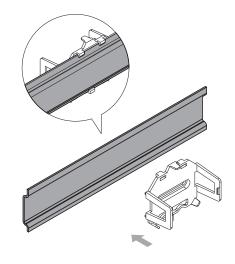
Step 1: Clip the mounting clip onto DIN rail.
