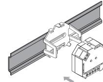
Step 2: Install the device onto the mounting clip in the correct direction.
